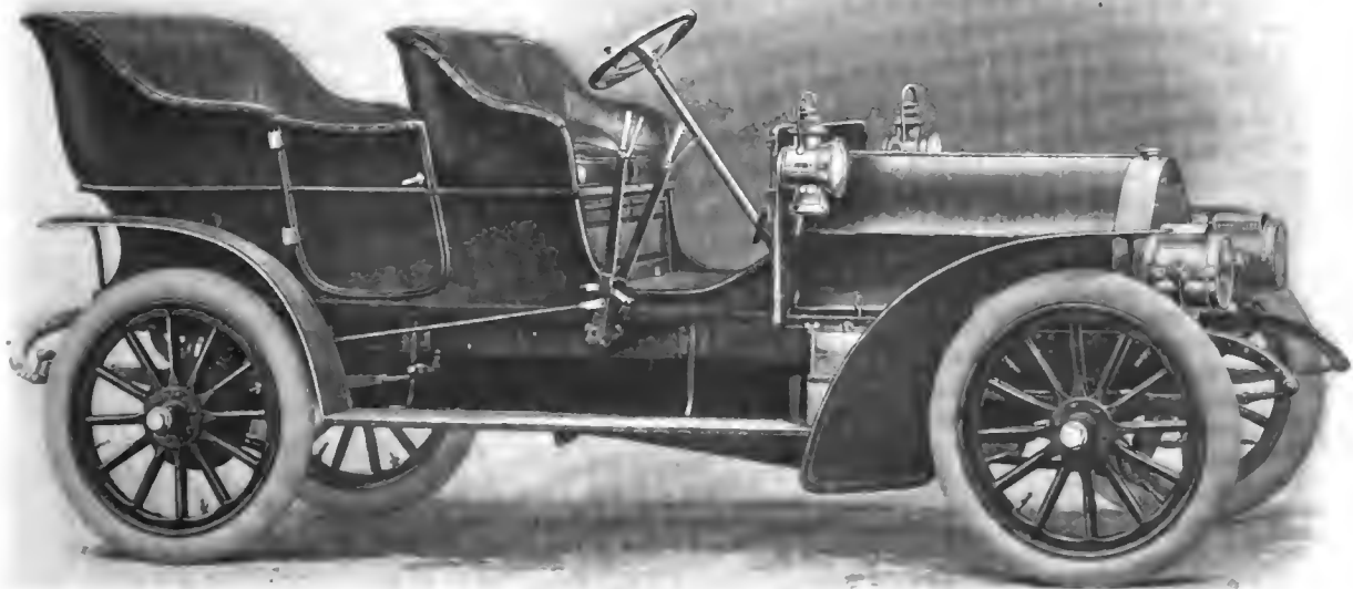
HEWITT TOURING CAR, 50 TO 60-H.P., 8 CYLINDERS, PRICE $5,500. Hewitt Motor Co., New York City.
